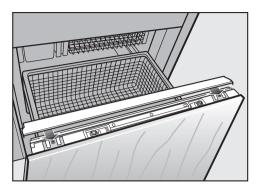
Insert the cover plate on the freezer compartment door.
